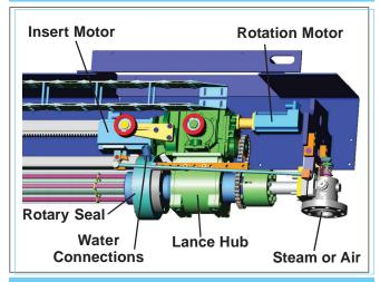
SmartLance<sup>™</sup>- A SmartClean<sup>™</sup> Product The SmartLance<sup>™</sup> is offered as part of Clyde Bergemann's SmartClean<sup>™</sup> Boiler Cleaning Optimization System. SmartClean<sup>™</sup> will make the decision which cleaning medium is best to use based on the actual cleanliness of the heating surfaces. The Multi Media SmartLance<sup>™</sup> is the most effective AND SAFEST cleaning tool available for heavy-plugging super heaters.
